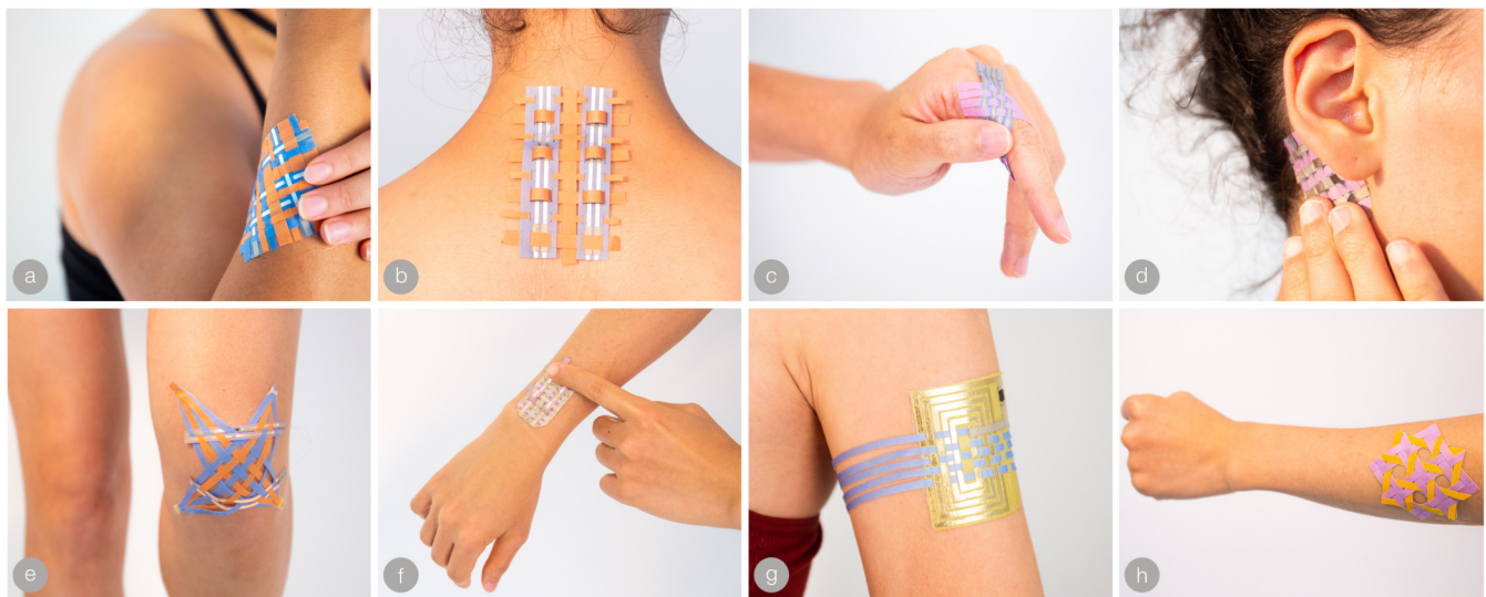
Figure 1: SkinPaper uses silicone-treated washi paper to weave lightweight and easy-to-fabricate on-skin interactions. Adopting a research-through-design approach, we contribute a design space with case studies that explore the variety of patterns, textures, and structures SkinPaper could afford: (a) A plain weave touch sensing matrix. (b) A protruded dome texture for LED diffusion. (c) A tubular finger touch sensing slider. (d) A behind-ear fuzzy weave touch input. (e) A 3D knee heating patch. (f) Collapsible textures as pressure input. (g) A twill weave NFC Tag with cut slits. (h) A double weave thermochromic patch.
