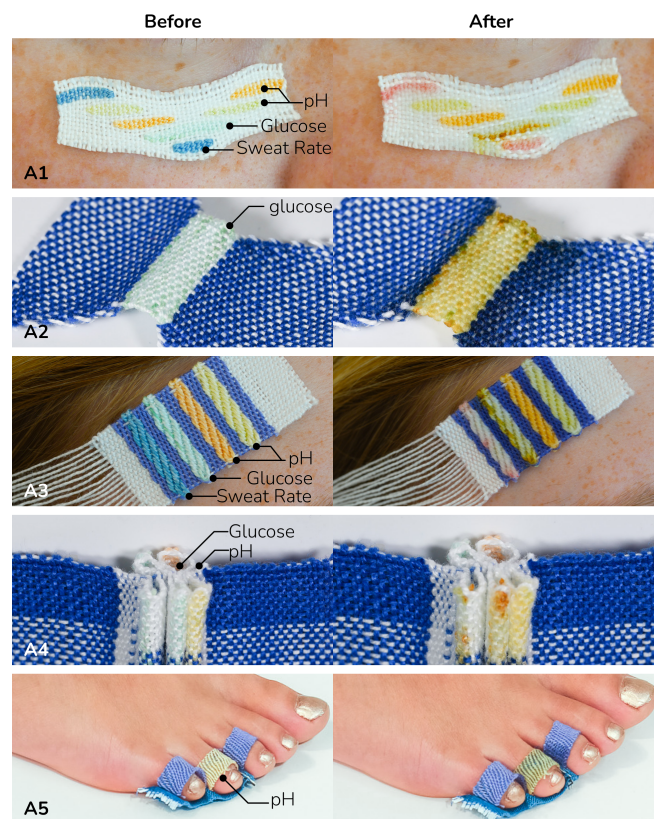
Figure 10: Close-up image of applications before and after colorimetric activation: (A1) Under eye cell patterned pH and glucose sensor, (A2) Under arm glucose sensor, (A3) Forehead and ear glucose sensor with floating warp, (A4) Between chest 3D pH sensor, (A5) Between toes pH sensor
